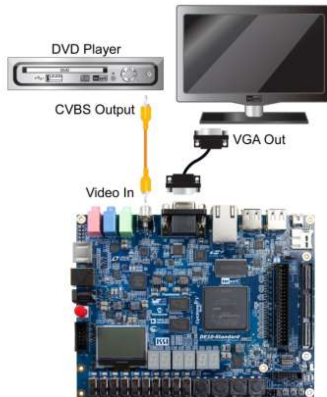
Figure 5-12 Setup for the TV box demonstration (VIP)
