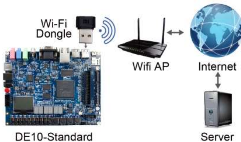
Figure 6-15 System diagram of USB Wi-Fi dongle
