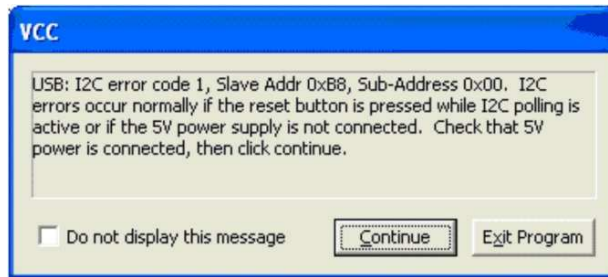
Figure 27. USB I 2 C Error Addressing Slave Address 0xB8
