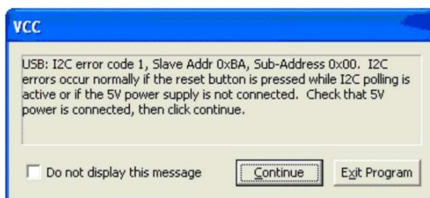
Figure 26. USB I 2 C Error Addressing Slave Address 0xBA
