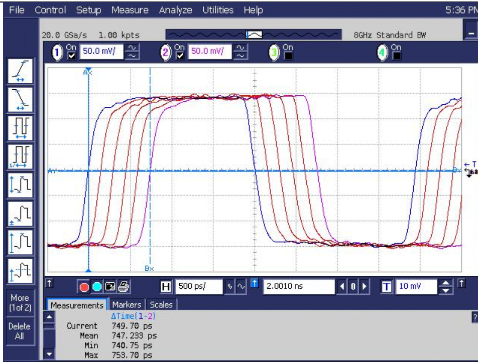
Delays from 0 to 2250 ps on CLKout1 referenced to CLKout0
