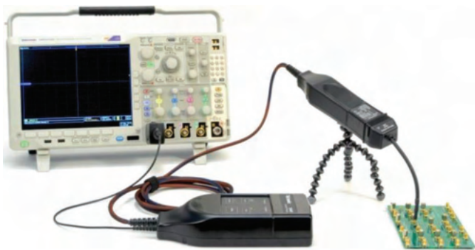
Figure 4: Tektronix IsoVu measurement setup.
