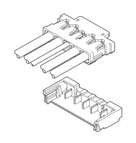
The AUH series is an SMT, wire-to-board crimp style connector that combines both power supply and signal communication into one connector system. It features an exceptionally low profile with a mounting height of only 1.85 mm and an overall depth of 5.2 mm in the mated condition. For such a compact connector, it offers an impressive current rating of 5 A.
