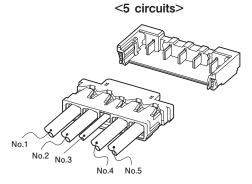
Power supply line: No.1, No.2, No.4, No.5 Signal line: No.3
