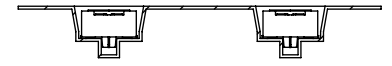
FIG 3 -TR: TAPE & REEL OPTION (MIS-057-01-X-D-K-TR SHOWN) (DIFFERENT AS SHOWN, OTHERWISE SAME AS FIG 1) (-076 POS MAX)
