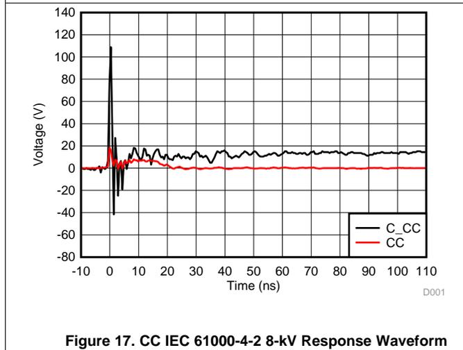
Figure 17. CC IEC 61000-4-2 8-kV Response Waveform
