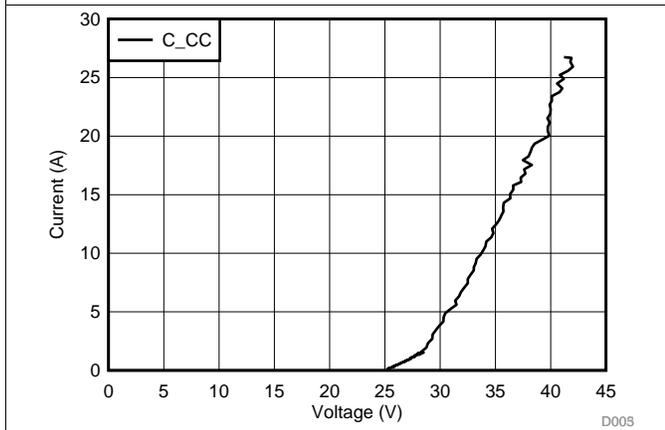
Figure 23. C\_CC TLP Curve Unpowered
