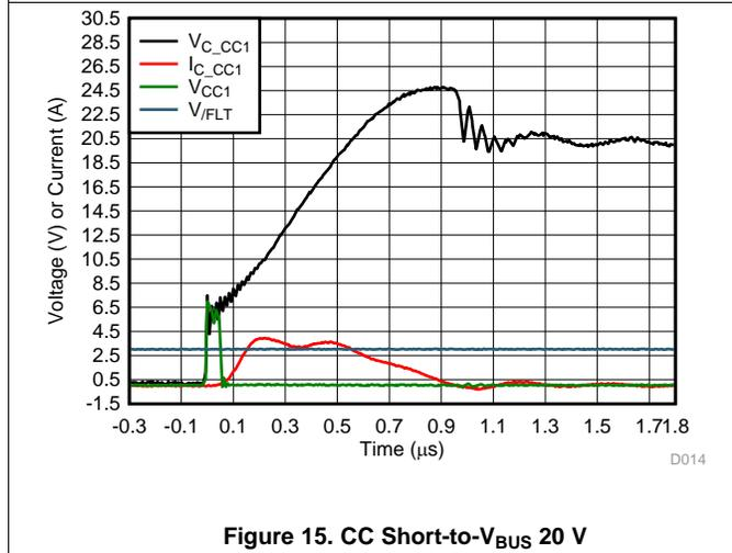
Figure 15. CC Short-to-V<sub>BUS</sub> 20 V
