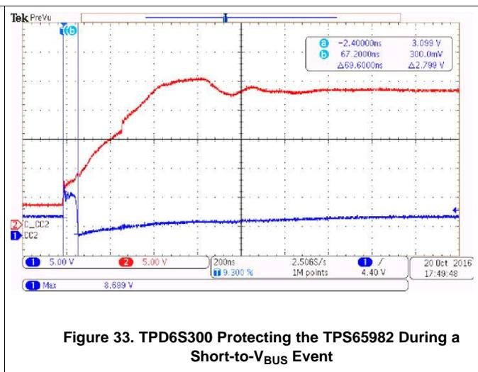
Figure 33. TPD6S300 Protecting the TPS65982 During a Short-to- $V_{BUS}$  Event
