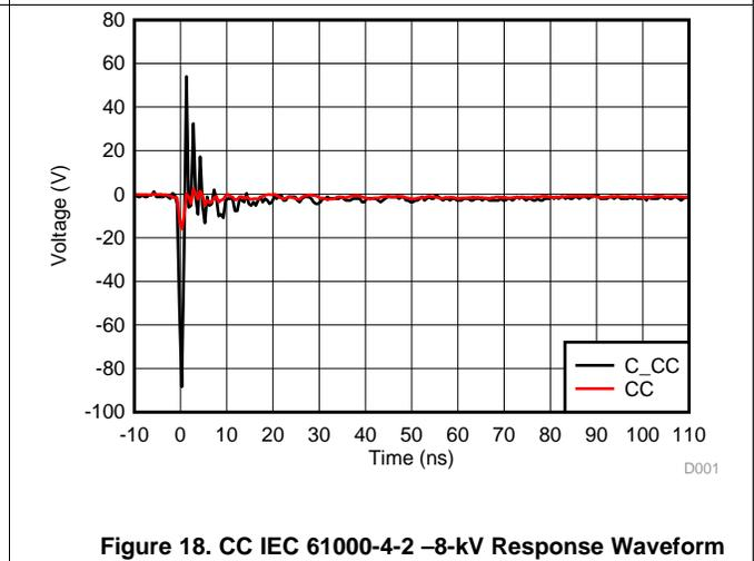
Figure 18. CC IEC 61000-4-2 -8-kV Response Waveform
