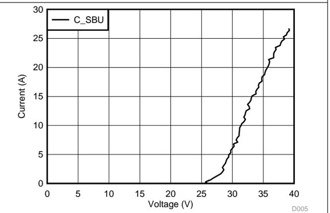
Figure 12. C\_SBU TLP Curve Unpowered
