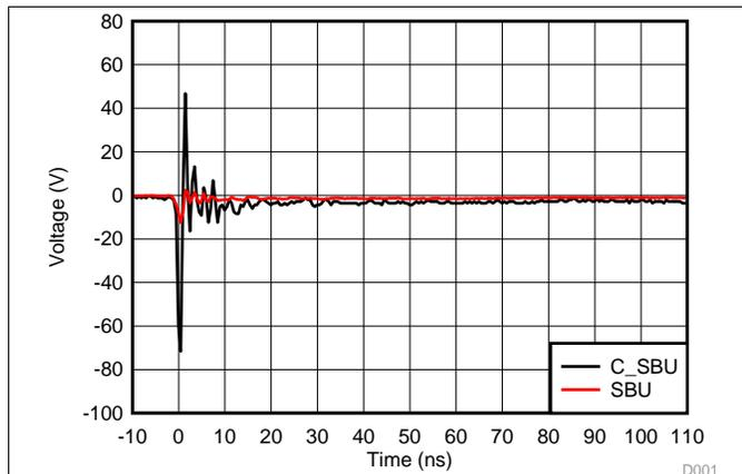
Figure 7. SBU IEC 61000-4-2 -4-kV Response Waveform
