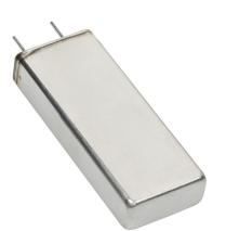
With a profile of 1.0" by 0.5" type MLSG Slimpack<sup>™</sup> capacitors fit into the tightest of spaces and meets a DC test of 5000 hrs at rated voltage, 125 °C. MLSG SlimpackTM is a perfect fit for military and aerospace applications requiring a low profile, rugged design and long-life. Specify type HRMLSG for high reliability burn-in.
