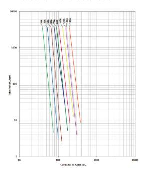
Note: FI = 1.00 (max. operating current :  $1.0 \times I_{rat}$  at  $23^{\circ}$ C)
