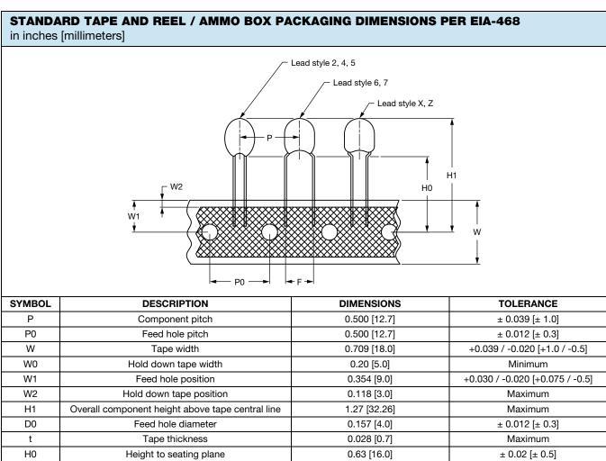
**Tape and Reel Packaging:** type 199D radial-leaded tantalum capacitors, all lead styles except 1, 3, and Y are available taped and reeled per EIA-468.
