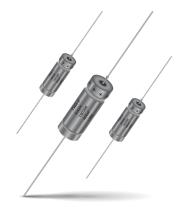
The TWA-X series represents a high temperature version of conventional wet electrolytic tantalum capacitors that are designed for use at 230°C. High capacitance cathode system allows high level of CV (Capacitance/Voltage) in standard case sizes.
