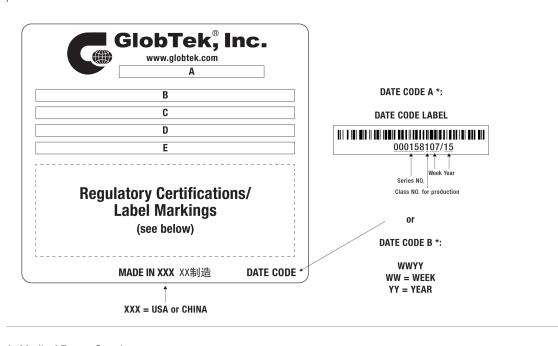
A=Medical Power Supply B=P/N: (料号) GTM91110P24036FSIM(R C=Model (型号) GTM91110P24036-FA-S D=Input (输入)100-240V~, 50-60 Hz, 4.0A E=Output (输出)36.0 V == 6.66 A, 240.00W
