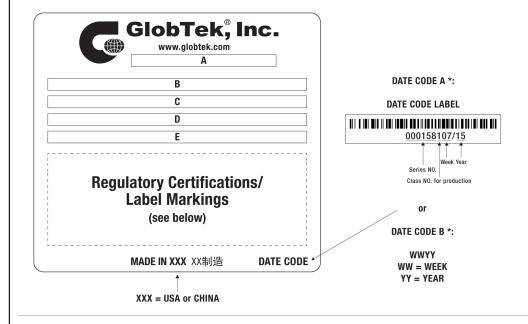
A=ICT / ITE / Medical Power Supply B=P/N: (料号) GTM43007-B6015-FW(R) C=Model (型号) GTM43007-B6015-FW D=Input (输入)100-240V~, 50-60Hz, 1.5A E=Output (输出)15.0 V === 4.0 A, 60.00W
