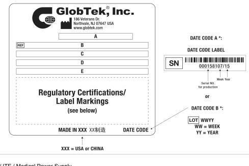
A=ICT / ITE / Medical Power Supply B=P/N: (料号) GTM43007-B6024-FW(R) C=Model (型号) GTM43007-B6024-FW D=Input (输入)100-240V~, 50-60Hz, 1.5A E=Output (输出)24.0 V == 2.5 A, 60.00W
