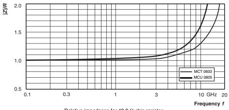
Relative impedance for 49.9  $\Omega$  chip resistor
