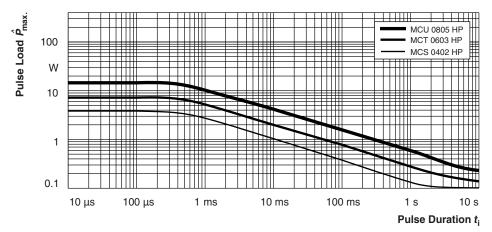
Maximum pulse load, single pulse; applicable if  $\overline{P} \to 0$  and n  $\leq$  1000 and  $\hat{U} \leq \hat{U}_{\text{max}}$ ; for permissible resistance change  $\pm$  (0.5 % R + 0.05  $\Omega$ )
