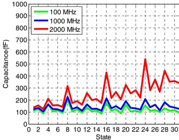
**Figure 7. Measured Shunt C vs Frequency**
