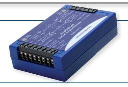
Model 485OP is an optically isolated RS-422/485 signal repeater. In addition to 2KV isolation on the data lines, it can be used to extend RS-422/485 circuits an additional 1.2 km (4,000 ft.), thereby doubling the range. An added benefit is the ability to add another 32 nodes to an RS-485 network and join 2 and 4 wire systems.
