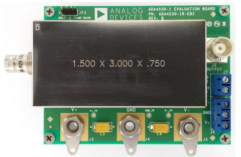
Figure 23. Evaluation Board Top View with SHIELD2
