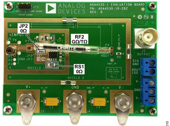
Figure 15. Transimpedance with Through Hole Feedback Resistor
