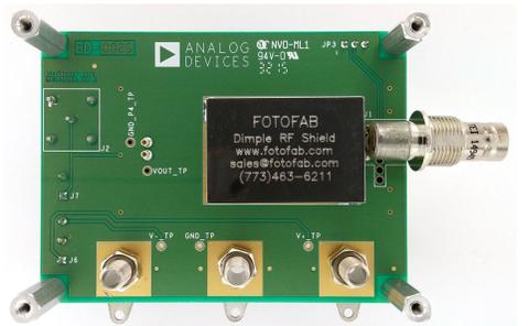
Figure 22. Evaluation Board Bottom View with SHIELD3
